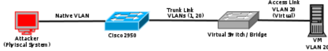
Fig. 6. Double tagging scenario where the attack is generated from a physical Kali 2.0 system connected to a Cisco 2950 switch in order to gain unauthorized access to virtual machines located on restricted VLANs within connected hypervisor environments.
