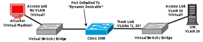
Fig. 4. Switch spoofing scenario where the attack is generated from a virtual machine connected to a virtual switched environment that has a physical uplink to a Cisco 2950 switch in order to gain unauthorized access to other virtual machines located on restricted VLANs within other hypervisor environments.
