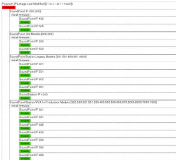
Now click the green **Enable** button under the **SoundPoint IP 335** and **SoundPoint IP 550** listings to enable them to be used when configuring an endpoint.
